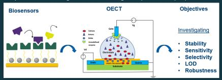
biocompatibility <sup>[2].</sup> However, OECT's high sensitivity leads to signal drifts due to changes in the surrounding environment such as pH effects, temperature changes, and interfering analytes. New
